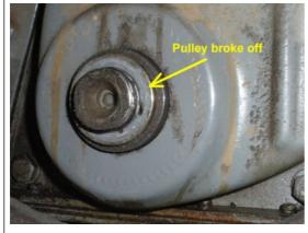
Crankshaft Pulleys or Crankshaft seals will fail over time. In this article we need to replace the Crankshaft pulley and the crankshaft seal behind the timing chaing. Here you see a typical pulley that has recently broken over time.
