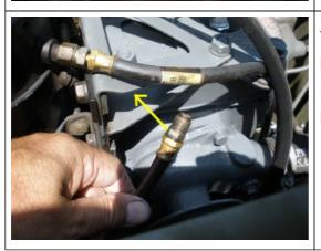
Tuck the oil line under the oil filter bracket, as gravity will cause oil to leak from the canister if it drops below the leave of the oil canister
