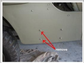
Prior to applying the stencil, remove any bolts or nuts so that the stencil can be applied on a flat surface (for best results).
