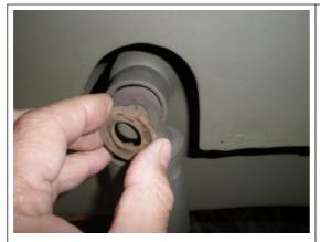
Now pull the washer off of the upper and lower pins.
