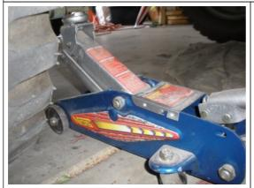
While replacing shocks may seem trivial, there can be some challenges geting the rubber bushings compressed in order to get the cotter pins on. While not necessary, we will take the wheel off in order to show you good pictures. First, we jack the rear driver wheel up.
