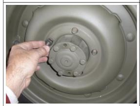
Next, remove the lug nuts and pull the wheel off.
