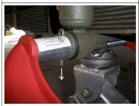
Once compressed enough, push the pin in. Note: you want to push the pin in as far as you can, because as soon as you release the C clamp the pressure on the cotter pin will not allow you to push it in any further.
