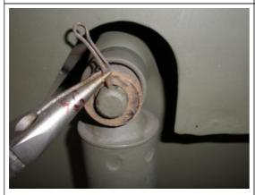
Straighten the cotter pin out on both the upper and lower areas and pull the cotter pin out.
