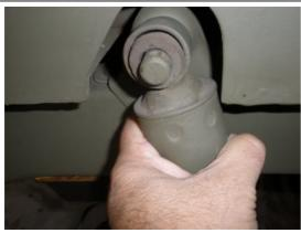
Next, wiggle the shock back and forth and the on the upper pin, and the shock will start to remove. Continue the same wiggle for the lower pin and the shock will pull off.
