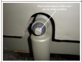
Use some emery cloth on the pins prior to pushing the shock/grommets on. Now, push both upper and lower legs of the shock on to the pins and push the grommets back to the fram as close as you can.
