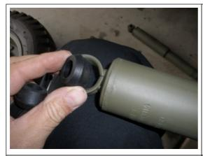
Next, prepare the shocks by placing the rubber grommets in both the upper and lower portion of the shock.
