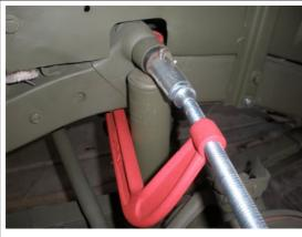
FRONT SHOCKS ?? The front bottom shocks can be applied like above, but what about the pesky top ? In this case, and 8 inch C clamp can work its way around the frame to apply the pressure needed to squeeze the grommets. BE SURE to do the top first on the front as well as back! Hope it helps!
