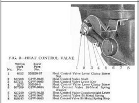
According to the TM's, the Heat Control valve is used to control the hot gases from the exhaust to help vaporize the fuel when the engine is cold. The counterweight arm you see here and the spring will react to the heat generated by the exhaust
