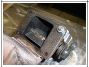
Here you see that the engine is cold and the counter weight is resting with the valve flapper in an open position on the inside of the manifold.
