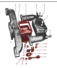
The Heat Control Valve, or Heat Riser on a WWII jeep was designed to help heat the intake air quickly in sever cold weather areas. Many jeep owners misunderstand the purpose of this component. First, the heat riser components that sit under the intake manifold and divert warm exhaust air. Components shown here.
