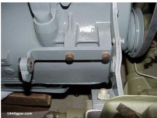
The generator bracket will have one rubber bushing, and secured to the block by two 3/8 x 7/8 -16 bolts.
