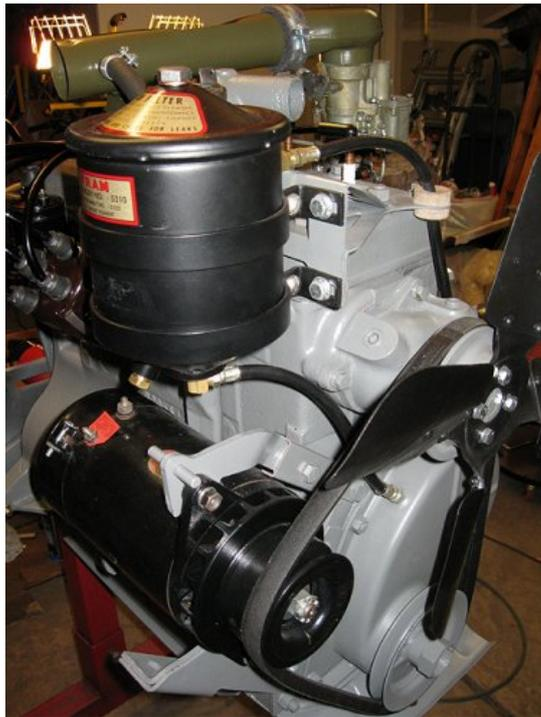
Finally with the generator around the fan belt, and arm holding the generator in place, you want to try and add the spring on the arm. Tighten the nut on the arm to generator and verify you have very little play in the fan belt. These wide belts don't need much tension. You should be able to deflect the belt about 1/2" with moderate finger pressure. Excessive tension is hard on water pump bearings. (tip from Pete Silfven) <br><br>Nice picture provided by Mike Strohlein
