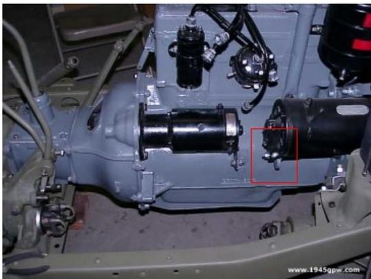
In this photo you can see how the generator fits onto the bracket. The bolts will insert from the inside, and the nut will be applied on the outside of the bracket. Note how the generator fits on the outside of the bracket.
