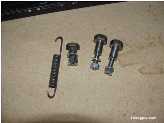
The two bolts to the right in this picture will be inserted into the bushing. Its a tight fit so you may want to grease the inside of the bushing with a little oil. Also when you insert don't insert all the way, because you have to lift the Generator into place first
