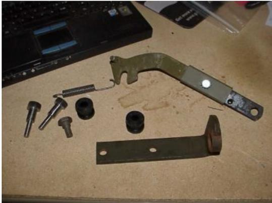
Installing your generator is not difficult, but the generator is heavy, so there will be some tough lifting times. To start with locate all the pieces needed in holding the generator in place. Adjustable arm, spring, bolts, rubber bushings and spring.
