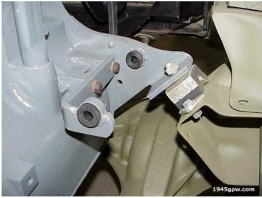
Install the 2nd rubber bushing into the hole in the block. You should see both rubber bushings.
