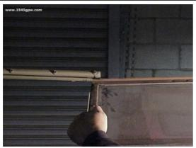
Remove the inner windshield from the windshield frame. The inner windshield slides out of the casing. I used a rubber hammer to help get it started. If its frozen due to rust, hit it with some penetrating oil, and tap it out
