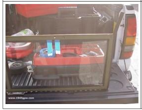
To hold the sealer tape in place, tape it down into place. You will cut all excess when bolted in. Press your top piece into place and install the bolts.
