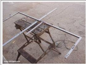
Next, I sand blasted the frame, primered and painted. Will install new rubber seal next, then the glass.
