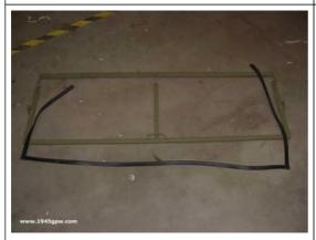
Now that the primer and paint are dried, I wanted to install the rubber seal that goes on the outside of the frame. I laid it out, and noticed that in order for it to fit correctly, it will need to be stretched.
