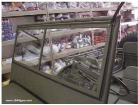
You see here, that the excess rubber seal needs to be cut as well. Wait till you install it back on the windshield frame, then you can see how much to cut off. I had about 3/4in additional to leave on past the frame.
