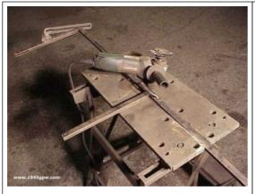
took my wire brush on the grinder and removed all the existing rubber seal in the groves, then I continued and removed the 4 layers of paint. I did this prior to sandblasting, so it would take less time in the long run.
