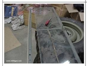
At this point, the top of the frame should just pop right off. You do want to be careful of any knicks in the glass you are removing as it can be sharp.
