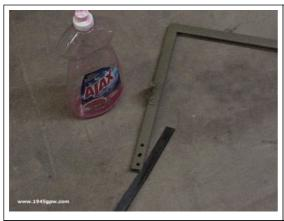
Use dishsoap to help get the seal to slip around the frame. I applied it, but turns out the seal slipped around pretty well anyway.
