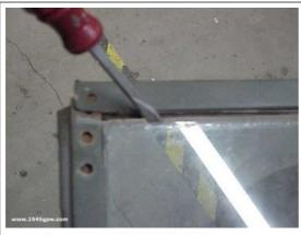
Once the screws are removed, the top frame should be loose. You can start prying it off. It should come off pretty easily, working it slowly.
