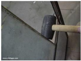
I pried it out far enough to start tapping it out with a rubber hammer. I kept tapping it out until I could pull the glass out. Repeat these steps to get the other piece out. I started rushing it and ended up breaking my other side, so go slow. If it is really tight, then squirt some penetrating oil around the glass frame.
