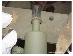
I added a new cork seal to the drive shaft. You can add a rubber one which will probably last longer, but I installed the cork one as to the specs. You have to place it on first before bringing the Yolk over the shaft
