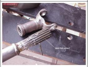
Once I got the ujoints out, I pulled the shaft apart and inspected the gold covering sheet that is on the inside. After further inspection, and this shim removed, it was obvious I needed to replace the front drive shaft. I located one from Northern California which was nice and tight.
