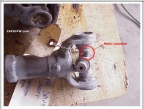
If you acquire a restoring project, you will most likely need to replace your u-joints. First, be sure you note where the location of your zerk fittings are (this picture shows the INCORRECT placement. the zerk should point toward the shafts). If you install these upside down they will be a bear to grease.
