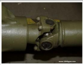
The installation of the ujoints is pretty basic once you get the cups installed on the clips side. Here you see it is a matter of tightening the U bolts on each side. Remember to keep the cups pressed on with your hand when installing. If they fall off, they will hit the ground and most likely fall out of place.
