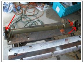
Tom Wolboldt tip: While installing your u joints, make sure your zerk fittings are all on the same side for easy lubricating. Otherwise, you have to turn your propeller shaft to lube.
