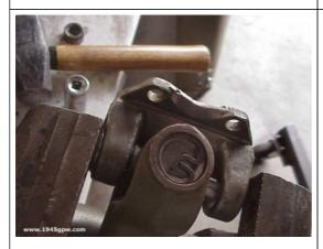
I shot some WD-40 in the rings of the yolks before trying to install. The cups will fit tightly, but they will give you resistance if you don't lube a little. Here you see on of the cups being pushed in with my Vise. I will repeat this process with the other side. NOTE: Keep your ujoint pushed into the cup so the bearing shafts won't move.
