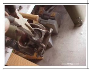
I used kneedlenose pliers to coil the clip, and pressing it into its slot. Once you have this one done, flip the shaft over and repeat the steps above
