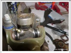
Pete Silfven Tip:Install the cups with the vise so they're flush, and then use a short socket to finish pushing them in. Do one side and install the snap ring, then do the other side. If the joint is tight, lay the cross across the vise again and tap the yoke to seat the cups against the snap rings. You'll notice that the hammer isn't used for installation except to free the joint up. This helps prevent any needles from being dislodged.
