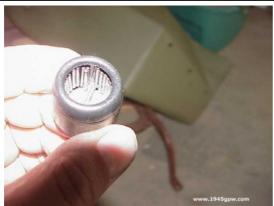
One of the common problems is installing the new rings and the cups fall off and the little shafts inside the cup fall out of alignment. I suggest to take all of the cups off before installing and install one at a time. Otherwise, you might run into this mess.
