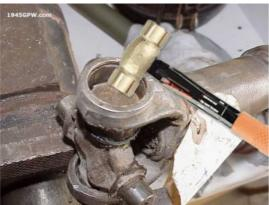
Once the rings are out, I put the shaft in a vise, and tapped the ujoint out by pounding out the spider ujoint. Use a Brass Hammer and a couple pounds and it will pop out. Make sure the clip is out on both sides
