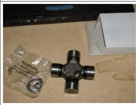
New ujoints come with the retainer rings and a zerk fitting. REMEMBER to install the zerk with it pointing toward the shaft, otherwise you won't be able to get to it. Also, you want to make sure that the zerks are lined up the same side on the shaft, AND, it is on the same side as the yolk.
