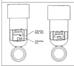
The range of adjustment is four turns. Look at the diagram, and see if you can push the bottom up into the key, and turn clockwise for firmness (rough roads), or counterclockwise for less.
