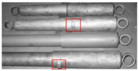
In order to rebuild your shocks you must have the type of shock that has a tab on the side of the main cylinder
