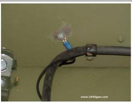
In order for the fuel gauge to read properly the sending unit must be grounded well. On the side panel you should have a clip there for routing your line to the fuel gauge. If you remove the paint and send your ground wire to this panel you should get a good ground.
