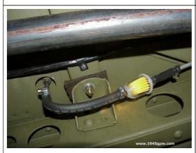
(Optional MOD). If you follow your fuel lines back to your tank you lines should marry up to the brass fittiing on the tank. Here you see a simple modification of adding an out of site fuel filter. Clear so you can see the sediment to change, but out of the way when people look at your engine.
