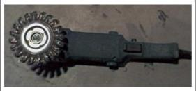
If you have a small item you want to remove paint you can get a wire wheel on your grinder and this will take the paint off. Using a wire wheel doesn't get all the way down into tough corners though.
