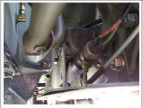
The brake light switch is a common point of failure. The brake light switch is found on the front of the master brake cylinder. There are two ways the brake light switch can fail. 1) pressing the brakes with the light switch on, and nothing lights up. 2) the brake light staying on when the electric light switch is on.
