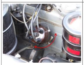
When you move the distributor one way or the other, you should be able to hear it run better as you approach the proper timing setting. The sound of the engine running should produce a consisitent "purring" when idling.
