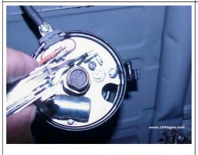
Once the arm of the points is sitting on one of the four corners of the distributor shaft, you can move the points in or out. With your feeler gauge find the .020 feeler, and check the gap. If you need more, then move the points open more, if less, move closer. Also, lube the cam shaft where the points touch lightly.
