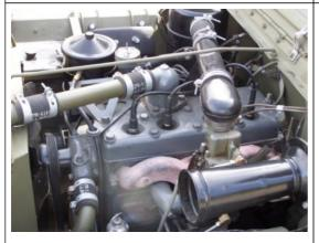
When the points, condenser, wires, and spark plugs have all been checked, then you want to check the timing of the vehicle. If your engine would start prior to your tune up, then it will probably work after you install these pieces. Try and start the vehicle. If it starts, get your timing gun out. If not, then go back to step one and start checking your gaps on condenser and plugs.
