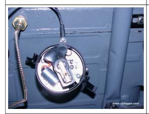
Inspect or replace the distributor points. If you replace them (inspecting for excessive arcing where the points come together), remove the screws holding the points on. Replace with the new points. To see the points clearly, remove the rotor.
