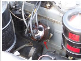
Adjusting the Distributor: Slightly loosen the distributor bolt into the block so the distributor can turn.
