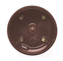
With the cap off, you want to inspect the bottom of the cap. You are looking for issues dealing with arcing. If you see damage to the cap due to excessive arcing, then replace the cap. If not, you may want to clean the cap inside and out.
