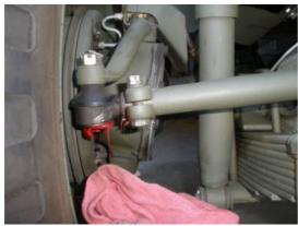
And last but not least, the front passenger side tie rod. Again, if you have a lot of grease, wipe it off. The more excess grease you have around the jeep the more grundge will collect. As you can see with these pictures, I need to go back and wash down from underneath.
