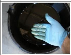
Now the last part. I drained my fluid on my transfer case side, so I need to replace that fluid. Before I do that, check the oil that was drained and check for metal fragments. If you find any have your transfer case checked by a professional. Otherwise your ok.
