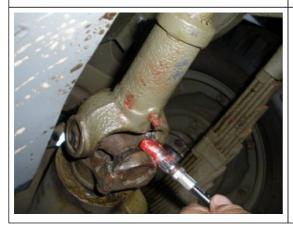
Scoot a little further under the jeep and locate your front drive shaft. You have two fittings one for the shaft going back and forth, the other one on the inside of the universal fittings. (you may need to turn the wheels for this one)
