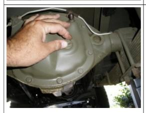
Now here, you have a choice to pack your wheel bearings. I just did mine on my restore, so they should be fine. If you have not, I would look to investigate them. Here we move to the back axle housing, and remove the plug and stick your finger into the housing and feel the 90w gear oil. Add if needed.
