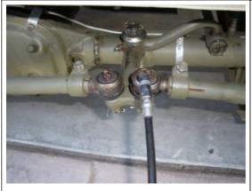
In the TM10-1513 I it also shows you the steps for lubing your vehicle. So between these steps and the manual from the link above you should be set to go. I start with the tie rods on the front of the jeep and move down the driver side and back around to the front on the passenger side. Here you see the two fittings for the Tie Rods, and I the third on the bell crank behind the tie rods.
