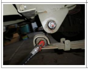
Moving around to the passenger side, grease the back spring shackles bolts
