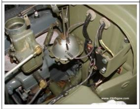
REMOVE HORN The horn will be in the way of you reaching the exhaust pipe and the oil line disconnect. Remove this and you will be able to reach these items.
