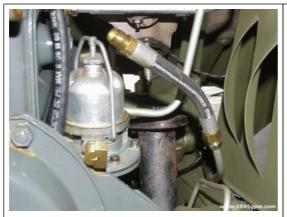
FUEL LINE DISCONNECT Remove the connection to the fuel pump. Here you see I have the late model which goes straight back to the fuel tank. Earlier models, line will go under engine to fuel strainer.
