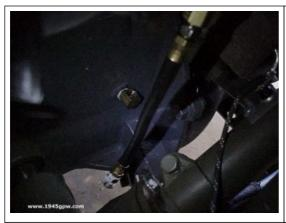
DISCONNECT OIL LINE: This line comes from the firewall. This can be removed from the tub on the tub, or at the block.
