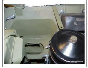
REMOVE BATTERY: You will need to remove some wiring, so disconnect the battery so you don't zap anything
