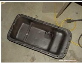
DRAIN OIL: This is optional, in my case, I drained it because I was replacing the rear main seal. So I removed the oil and the oil pan.
