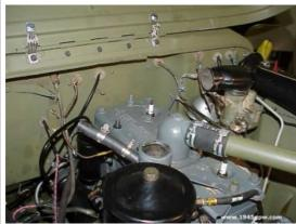
REMOVE AIR FILTER TUBE: I removed this so that I don't screw it up while hoisting.
