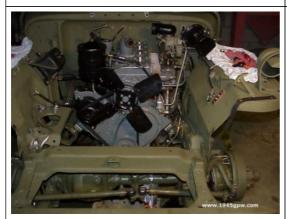
REMOVE RADIATOR: Remove the connections for the upper and lower tubes. There will be two bolts to remove on the bottom.
