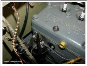
REMOVE COIL WIRE: this wire comes from the firewall, so you will need to remove it. As well as the cable to the distributor cap (if you take it off like I did.)
