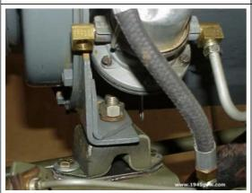
leave the engine mounts secured to the engine and unbolt them from the crossmember. It makes it a lot easier when reinstalling the engine because you don't have to line the mount studs up at the same time you're trying to line up the clutch splines. (tip from Pete Silfven)
