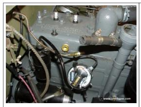
DISCONNECT TEMPERATURE GAUGE: Cable comes out of the firewall, so be sure this is removed from Head.
