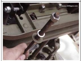
REMOVE STAY CABLE and CLUTCH HOUSING BOLTS: Many jeeps don't have the stay cable, if you do, disconnect it.
