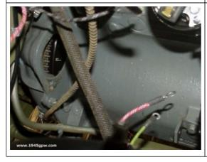
DISCONNECT STARTER: Remove starter and wires
