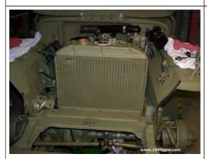
(OPTIONAL) Remove Grill: If you decide to remove the grill, Its actually easier than I thought. Disconnect the wires on the driver fender junction, and disconnect the bolts to the fenders and frame.
