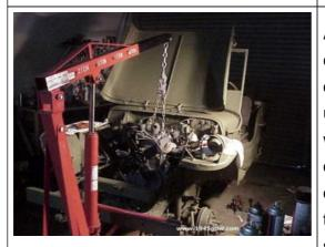
At this point, your bellhousing connection is ready to be disconnected. Be sure to have a jack under the bellhousing to support the weight as the engine is being pulled out the front. In my case, I will pull it out about 2 inches in order to allow the crank to drop and I can get the seal back on.
