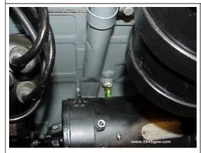
DRAIN RADIATOR: To start your engine removal, we start with draining the Radiator fluid from the block. While this is draining, continue with the other steps, as this will take about 20 minutes.
