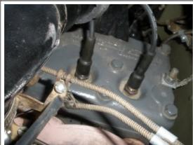
Remove the linkage for the Choke and throttle cables. You might need to pry the holder a bit to let the choke cable free.
