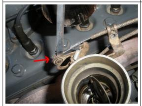
Loosen the throttle screw.
