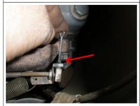
Install a new cotter pin to the gas pedal linkage. Insert and seperate the ends of the new cotter pin with needle nose pliers if needed.
