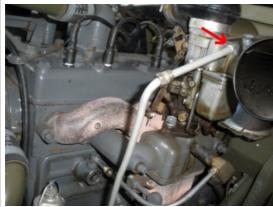
Remove the Fuel line from the carburetor
