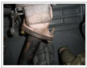
Add a new exhaust gasket to the exhaust flex pipe and tighten the bolts into the bottom of the manifold.
