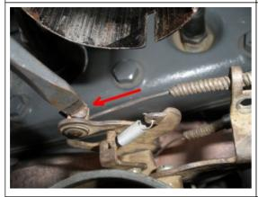
Install the throttle line back into the insert and tighten the screw down.
