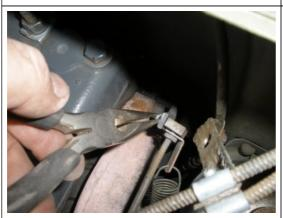
Remove the cotter pin from the gas pedal armature. Note: it is a good habit to replace cotter pins after removing them.
