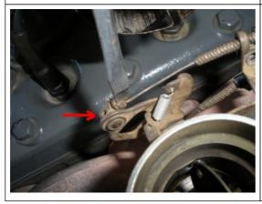
The throttle cable will slip out of the screw holder.
