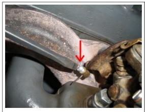
Install the choke pin at bottom of linkage. Insert the choke line through the pin and tighten the screw.
