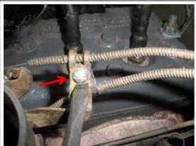
Install the choke and throttle line holder connection. Note: you may have bent this out a little when removing, you should crimp it back a bit to hold the throttle cable (top) firmly.
