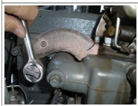
Locate each of the nuts on the intake/exhaust manifolds, and remove the bolts.
