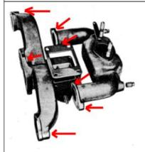
Removing the Exhaust takes a number of steps because there are many other linkage disconnects that need to happen as well. Note here the seven primary nuts that need to be removed from the intake/exhaust manifolds
