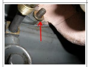
Just a note, be sure you have the correct washer on the two piece connections under the manifold (where intake and exhaust come together). Tighten all the nuts on to the manifold, all seven!
