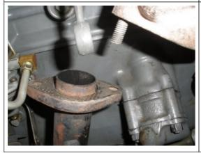
Disconnect the Exhaust flex pipe from the manifold. Note: watch for the gasket.
