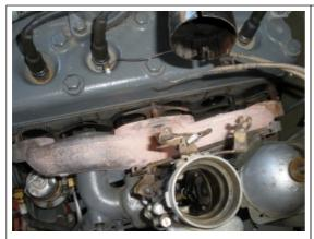
At this point, tug on the manifold a bit and it should seperate from the block. It is heavy so it might take a decent tug. Try not to strip the bolts on the block on the way out.
