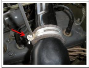
Finally, pull your seal back from the air horn back over where the two peices meet, and tighten down. You have now reinstalled your manifold!
