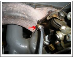
Loosen the choke screw and slip the pin out so the cable is free.
