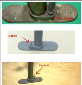
At the base of the pump there are some differences in where the valve has been positioned. Each manufacturer decided on placing the valve at a different position.<br/>
