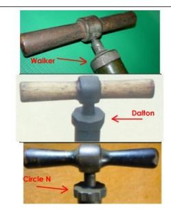
There are a couple of distinguishing features between pumps. Starting at the top of the tube. The type of cap is different among the manufactures.<br/>
