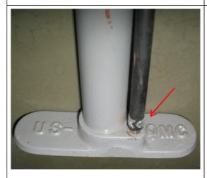
Lets first look at the Tire Pump introduction to MB's. The first tire pumps were added to the bottom of the rear seat of MB's about May of 1942 and were the QMC grey color pumps. According to Nabholtz, the QMC pumps were continued on MB's until Sept 1942. These QMC pumps did not include the Air Chuck as part of the Parts list. Part is listed as WO-A7511.<br/>
