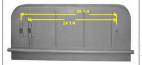
Now lets look at the air pump bracket under the rear seat. There are two possible lengths that have appeared on WWII Jeeps with a difference in the length on the bottom of the rear seat as shown. It is unclear when the differences showed up on productions lines, but most likely later in production. More research is needed to see if these sizes were both for MB's and GPW's, or just MB's.
