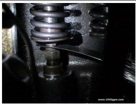
Here is a close up of what you are checking the gap on. According the the TM the gap should be .014 when cold for both intake and exhaust.
