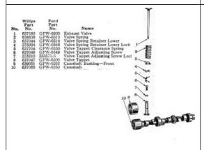
(TIP by Pete Silfven) Adjusting valve clearance when the tappet is worn cupped and it can't be done with a feeler gauge. The tappet thread is 24 threads per inch. To find out how much the tappet adjuster moves in one revolution, divide 1.000 by 24. This gives a movement of almost .042" per revolution.
