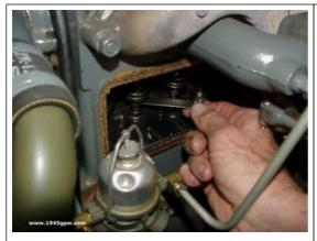
Here you see I am checking the gap of the valve in Cylinder 1 intake.
