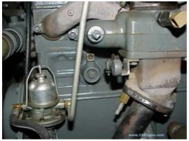
Valve cover installed back on.
