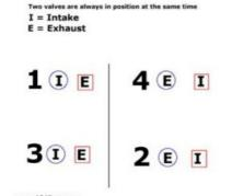
Now, if you think about this, you have 8 valves. 4 are intake, and 4 are exhaust. There are always two valves in position at the same time. The diagram below helps explain this. For example, If I want Cylinder 1 Intake valve to be closed (so I can check the gap .014), then Cylinder 4 Exhaust is in the same position and I can check it. Therefore, you can check two valves with each crank position.
