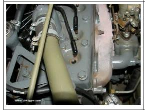
In order to adjust the valves they have to be in a certain position, so turning the crank will be necessary. I removed the spark plugs to make that an easier chore.
