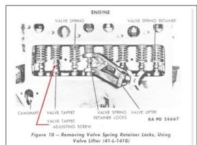
on the adjuster screw, so we divide .042 by 6, and get .007" per flat. Now, with the cam in position to adjust a particular valve, unscrew the adjuster to the point where the tappet just quits revolving freely This is zero lash. Then screw the adjuster in the proper number of flats to get the correct clearance. For .014", that will
