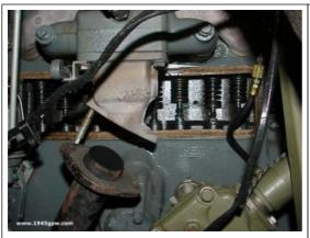
Ok, now that the cover is off, I removed the PCV line and the exhaust pipe which allowed me to get the cover out. I wiped down around the cover, and made sure I didn't have any drips.
