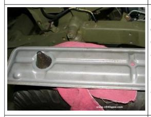
After each pair of valves get (from diagram above) get verified, turn the crank to the next pair as shown in the above diagram, and repeat the steps. I finished mine in about 1 hr. I needed someone to hold my LED pen light and to turn the crank, so it will help to have a friend.
