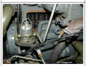
Here you see the cover popped off. Gasket still looks good, but how do I get the valve cover out? I removed the PCV line and disconnected the exhaust pipe as well.
