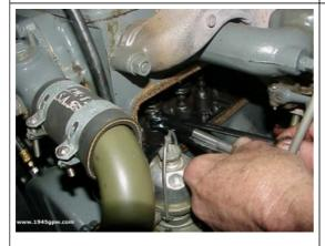
To adjust these, you will need two 1/2in open end wrenches. In my case, I had a bigger gap than I wanted. You place one wrench on the tappet (bottom) and one wrench on the top nut. Then you separate the wrenches to make the gap more narrow. In my case, I needed to bring go from .015 to .014. When I make the adjustment, I check again with the gap tool.
