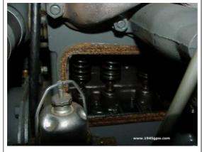
It doesn't really matter the order of the valves you are going to adjust, so you can start with any of them in the closed position. The tappet will be all the way down when closed. Have someone turn the crank (clockwise) until your designated valve is in the down position.
