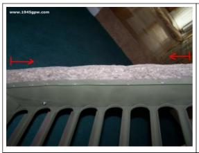
I stapled the ends of the complete felt piece first, then worked into the middle. This helps the felt stay in place and keeps it from buckling in between staples. Once you get a couple of them in, it starts to go pretty fast.
