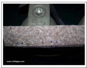
After each hole was created, I marked it with a felt pen. After you create the hole it is hard to find it.... so I marked the hole so I know where to place the staple when needed.
