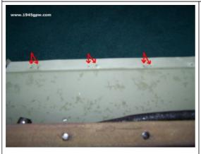
My impression of installing radiator felt was much different that what the actual effort needed. I thought simple, push staples through felt and clamp down. I also thought I could do this with the grill on the frame. Wrong. You will need, large pliers, Needle nose pliers, and an Ice pick or nail. Unless you have a repo grill, your staple holes should be present on your grill.
